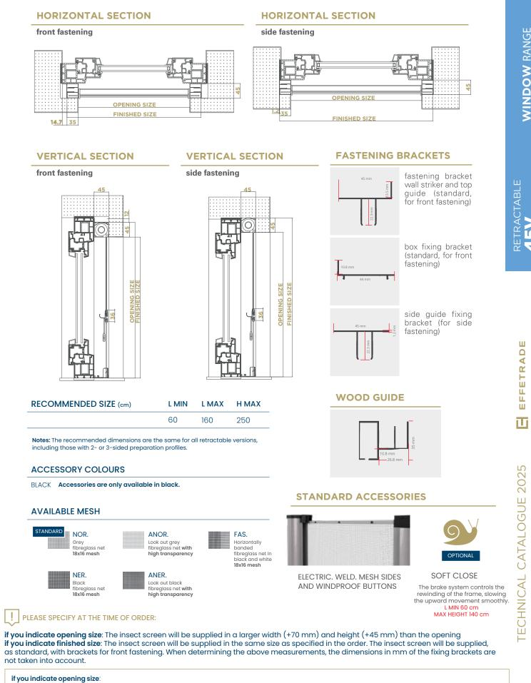
RECESSED 45V WOOD GUIDE The insect screen will be supplied in a larger width + 70 mm and in height + 45 mm
