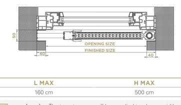
opening size The insect screen will be supplied in a larger width (+ 80 mm) and height (+ 65 mm) than the opening if the finished size is indicated The insect screen will be supplied
