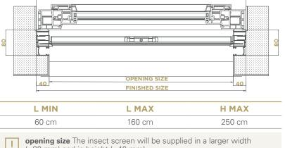
(+80 mm) and in height (+40 mm) if the finished size is indicated The insect screen will be supplied in the same size.
